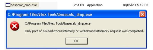
This is because of the alignment issues mentioned earlier - the filesize has also increased as a result. Open the app in LordPE and look at the sections. The raw offset and raw size values are wrong. We will have to make the Raw values equal the Virtual values for each section for the app to work. Rightclick the UPXO section and select edit header:
